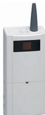
Do not forget that because it is a media coupler, it has a table of filters by default it is empty and activated, so it will not pass any group address until the table is configured in the same way as a line coupler.
