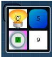
In the example on the left, the matrix element has been configured for 4 values (0, 5, 7, 9). Each field has an individual design. Press the control element to open the matrix field and press the required value setting button.
