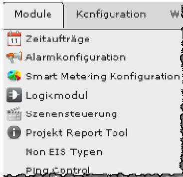
CBS Evolution offers the user numerous functions to automate and monitor an installation. The functions are structured in module form and can be configured via the main menu *Module*. In addition to the basic configuration of function modules you can also modify the configuration in the visualisation.
