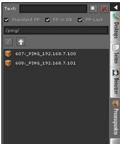
A process point is automatically generated for each device that is to be checked so that the device status can be easily linked to the alarm management or the visualisation. The process points are listed in the process point selection list in the *ping* folder. The process point name is formed according to the following order *\_PING\_<ip>*. The data type is DPT1. A 0 is sent if the device is not available and a 1 when it is available.
