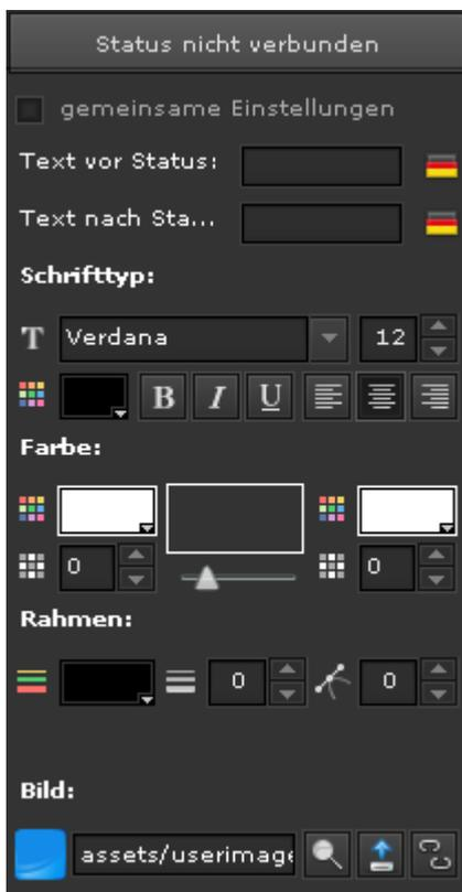
The number of configurable status types depends on the component and is shown in separate properties sections (e.g.: **status not connected, first status, second status, status connected**). The display options and configuration parameters are identical for each status, so that the following description for **status not connected** equally applies to every other status. Component-specific attributes will be explained together with each component.
