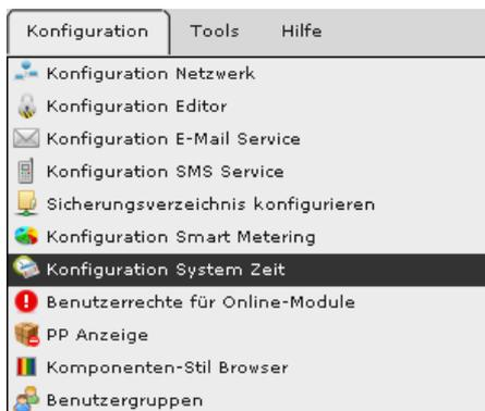
To ensure that weekly and annual schedules work correctly it is essential that the CBSE server is configured with location-specific time and date settings. Use *Configuration/System time* to load the configuration dialogue.
