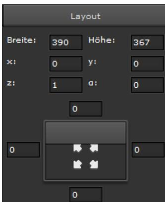
By default, the frame and page size are adjusted to the size of the window. If you want to create individually sized frames in a window, go to the properties menu "Layout" and select the required settings.
