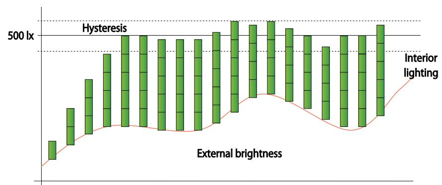
c.ii. The brightness sensors that are used for CLR should have a measured-value resolution not more than 15% of the set point value. Ex. set point = 600 lux; tolerance < 90 lux.
