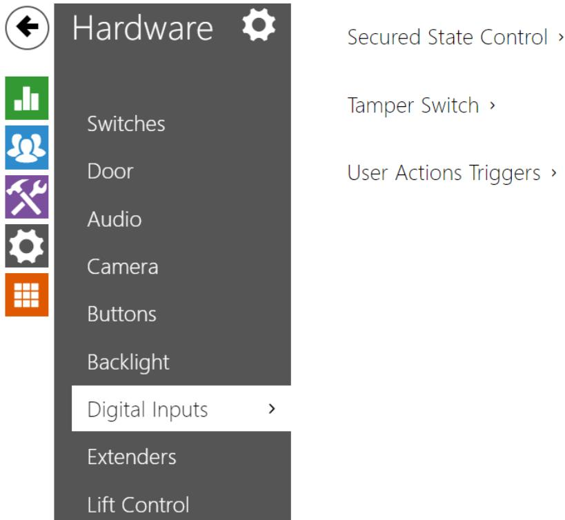
In this configuration section set the parameters associated with digital inputs and their interconnections with other intercom functions. The digital inputs are available in selected intercom models or where appropriate equipment is installed (e.g. card readers).
