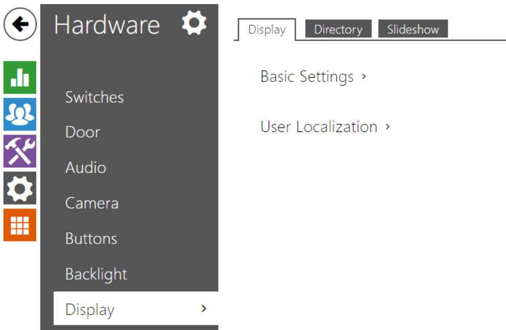
Some intercom models (**2N® IP Vario**, **2N® IP Verso**) can be equipped with a color LCD display. The device state is displayed (call progress, door opening, etc.) and the following modes are available:
