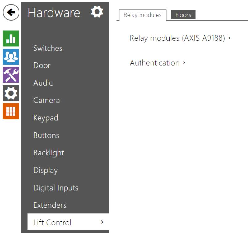
To control the floor lift access, connect the AXIS A9188 relay module to the 2N IP intercom (**2N® IP Style, 2N® IP Verso, 2N® IP Force, 2N® IP Safety, 2N® IP Vario**). Up to 8 relay modules can be connected to one 2N IP intercom, each of which can control up to 8 floors, which makes a total of 64. Make sure that the IP intercoms Lift module license is active (Part No. 9137916) to make this function work.
