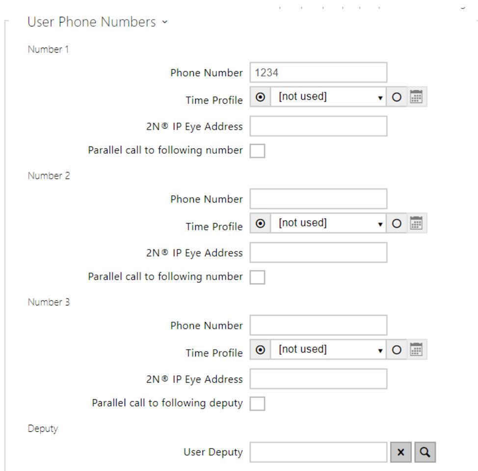
You can also use the **2N IP intercom** with one or more IP phones without a SIP server. Use the Direct SIP Call. For outgoing calls and enter the called phone SIP address (sip:phone\_number@phone\_ip\_address) instead of the phone number.
