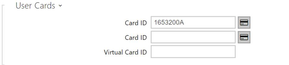
Each of the intercom users can be assigned two access RFID card.
