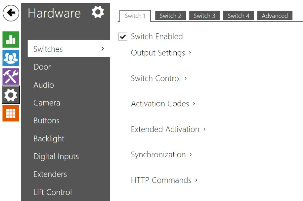
Switches provide a very flexible and efficient control of such intercom peripherals as electric door locks, lighting, additional ringing signalling, and so on. **2N IP intercoms** allows you to configure up to 4 (depending on model types) independent all-purpose switches.
