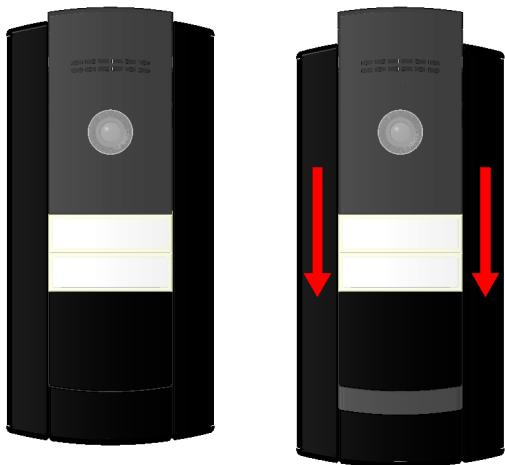
Frame Demounting. First use the torx handle enclosed to remove the screw that fits the frame to the **2N® IP Base** structure.
