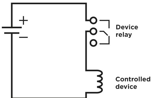
Wiring diagram for the controlled device's electric circuit closing
