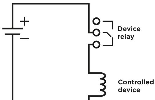
Wiring diagram for the controlled device's electric circuit opening
