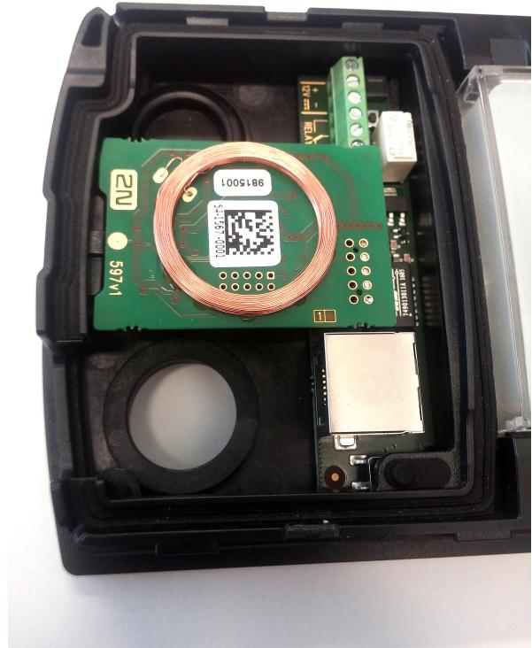
3) As the last, it is necessary to fix the module using tabs built into the structure of **2N® IP Base**. This tab is highlighted in the following picture by the red rectangle.
