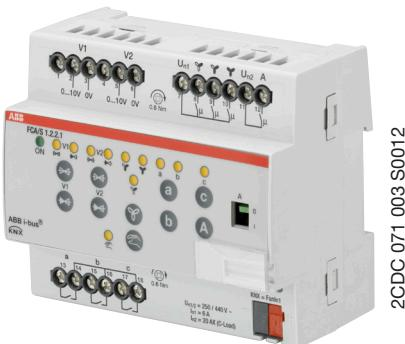
The Fan Coil Actuator FCA/S 1.2.2.1 is a modular installation device (MDRC) in Pro M Design. It is intended for installation in the distribution board on 35 mm mounting rails. The assignment of the physical addresses as well as the parameterization is carried out with ETS.
