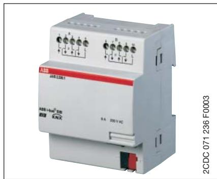
For controlling 2 independent groups, each with 2 shutter drives via ABB i-bus® including the functions Up/Down, Step/Stop, Move to position, Sun protection automatic control and Heating/cooling automatic control.
