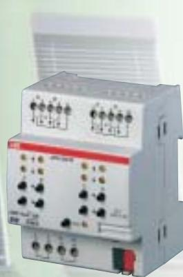
Shutter Actuators with manual operation ensure increased **operational reliability** in the ABB i-bus® EIB installation. The connection of the motors can be tested at the wiring stage, even without bus voltage. During the commissioning, the parameter settings are easier to test using direct operation and the blinds and ventilation can continue to be controlled in the event of bus voltage failure or other disruptions.
