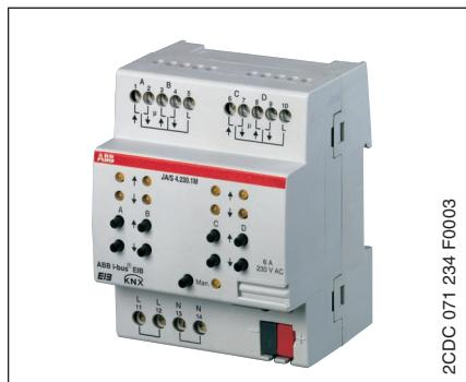
The Shutter Actuator JA/S 4.230.1M is used to control a maximum of four independent 230 VAC drives for positioning shutters, blinds, awnings and other hangings as well as for controlling doors, windows and ventilation flaps.
