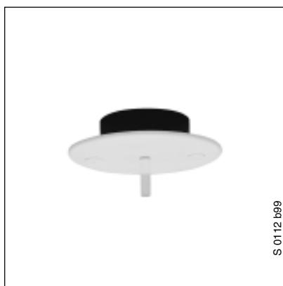
With the light sensor, it is possible to determine the brightness level in closed rooms. The light sensor is mounted in a standard installation box in the ceiling. The cover (white) of the sensor is stuck firmly onto the device. The complete unit is then screwed into a flush-type box.
