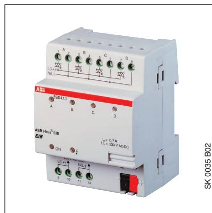
The 4-fold electronic switch actuator is a DIN rail mounted device for the static switching of resistive loads. The device is suitable for installation onto a mounting rail in electrical distribution boards or panelboards for heating systems. The connection to the EIB is established via a bus connection terminal.
