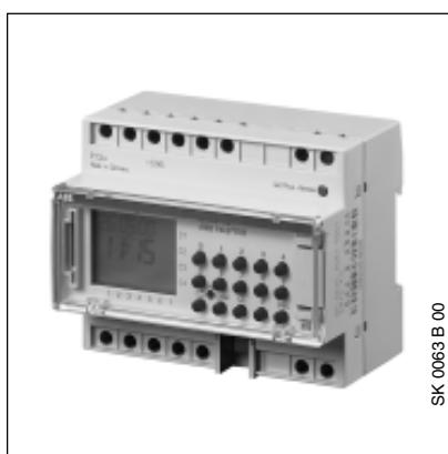
The 4-fold week time switch with a day, week and year program is a DIN rail mounted device for insertion in the distribution board. Connection to the EIB is carried out via the bus connecting terminal at the front of the device.
