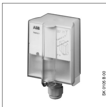
The antenna is used in connection with a radio-controlled time switch for receiving the time standard of the DCF 77 transmitter located in Mainflingen near Frankfurt. This time signal is transmitted via radio and can be picked up within a radius of 1000 km around Frankfurt.
