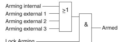
The system can be armed via the first "Arming" object, the second object or the third. The inputs are linked with an OR function. In addition, an "Activate arming" object is enabled via a corresponding parameter. If the object is visible, arming is enabled with an ON telegram. An OFF telegram disables the possibility of arming the system.
