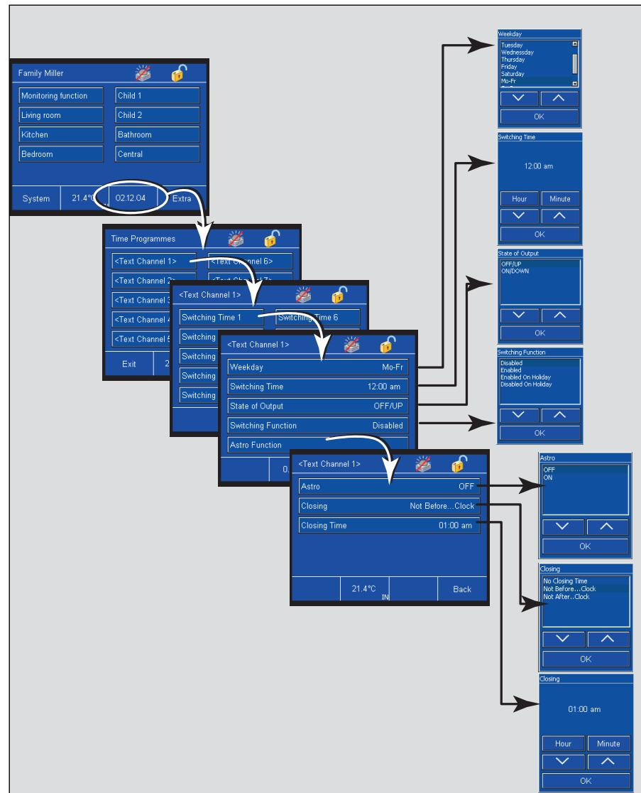
The switch channels of the SMARTtouch panel have 10 (5 for LEANtouch) switching times each. The switching times can either be set on the panel (see diagram) or in the parameters of the panel software.
