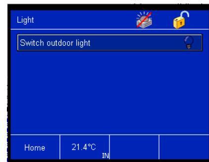
The “Name of touch surface” is always on the left-hand side of the touch surface. This can be freely assigned to each touch surface with the corresponding parameter.
