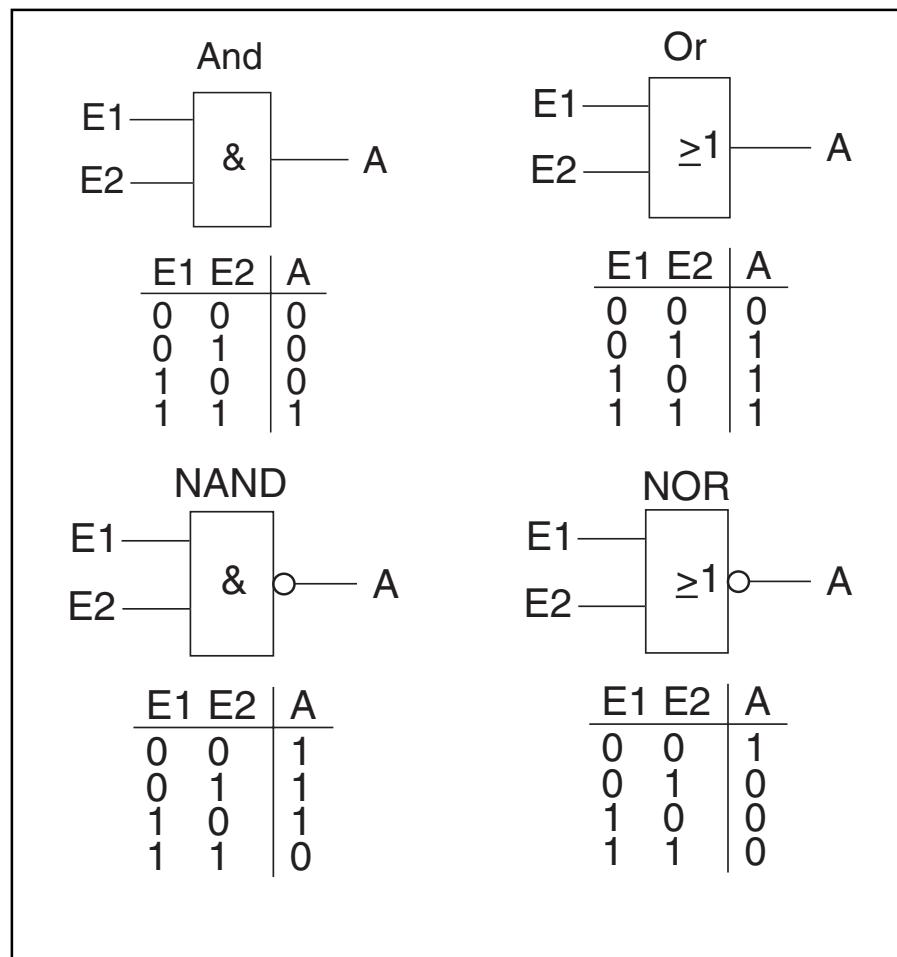
Up to 20 different logic functions can be integrated with up to 10 inputs in the panel. Each logic function can adopt one of the following functions:
