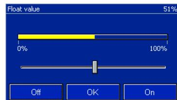
If the "Floating value" touch surface is pressed, the panel displays a slide rule and three buttons in the open window. Values can be set intuitively via the slide rule by adjusting the control button. Depending on the setting, the value can be increased or decreased via the buttons. The values will be sent out directly during the operation of the slide control.
