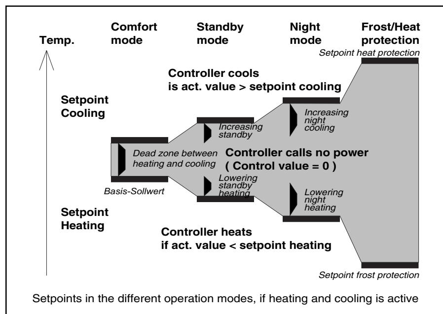
so, a 2-byte temperature value must be sent to the object "Base setpoint".
