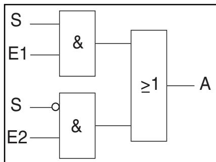
Via the "Multiplexer" logic function, the input data to the output can be controlled directly. The function has four communication objects "Controller", "Input 1", "Input 2" and "Output". The diagram above indicates the function of a 1-bit multiplexer (S=Controller, E1=Input 1, E2=Input 2, A= Output).
