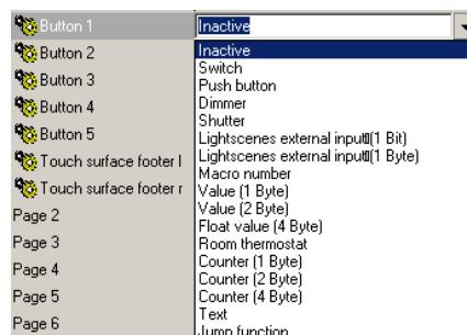
The parameters of the individual functions are displayed on the right-hand side. The parameters of the function
