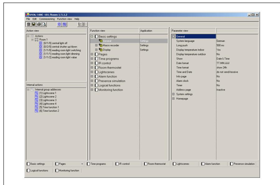
The functions and applications are arranged with all the communication objects in the centre. If necessary, the individual functions/applications must first be activated so that the communication objects become visible. The functions are defined via a pull-down menu.
