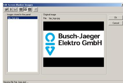
To do so, select the required file via the "Open" symbol - graphics files of the type \*.jpg, \*.bmp or \*.gif can be imported. The graphic is then displayed in the preview window. The image is prepared for storage in the panel via the button "Save background image in the panel".
