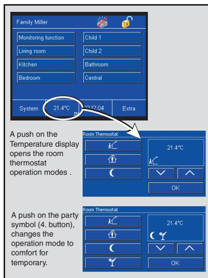
The LEANTouch/SMARTtouch panel has an integrated room thermostat. This has a comparable functionality to the usual EIB room thermostats.
