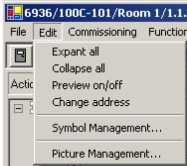
If the function "Manage images..." is retrieved from the "Edit" menu, a dialog window opens via which the images can be imported into the panel software.
