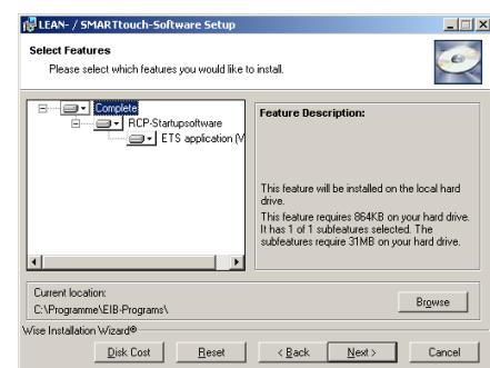
In the "Select functions" dialog, you define whether the VD2 or VD3 files should be copied locally onto the hard disk. You require these to be able to use the LEANtouch/SMARTtouch panel in connection with an ETS version. (Also observe the note at the end of this chapter).
