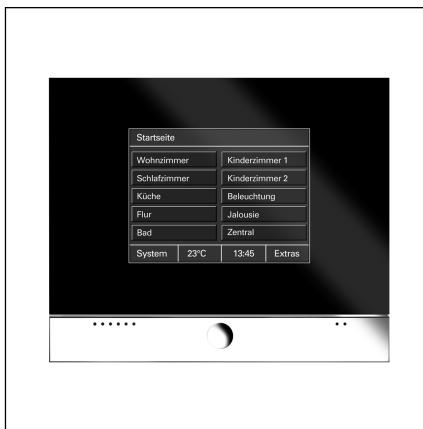
The SMARTtouch panel is a high-quality EIB touch-sensitive display. The panel offers approx. 210 operator functions with a monochrome display. It is used as a control, monitoring and indication unit for the complete EIB installation which can be operated across different rooms.
