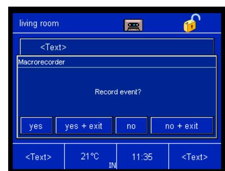
In the "Save macros" mode, the panel displays a dialog after each executed function in which the user can define whether or not he wishes to save this function in the macro. At the same time, he can finish the storing of macros in the same window. Up to 20 functions can be stored in a macro.
