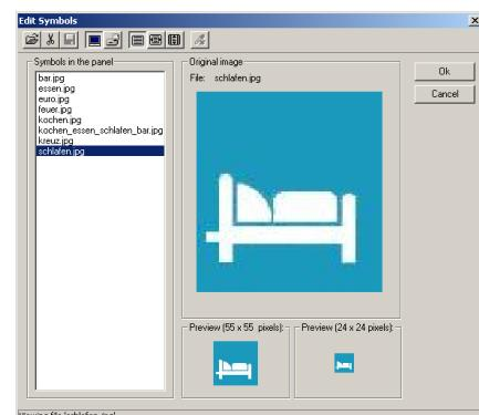
In a similar way to the function of importing background images, various graphics files (\*.jpg, \*.bmp or \*.gif) can be imported via the "Open" symbol in the "Manage symbols" dialog window. The panel software can manage a total of 126 different files.
