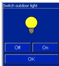
If this button is "Active", a window opens when the touch surface is operated. The "Name of touch surface" appears in the window as a heading. The buttons (designated here with "ON" and "OFF") can be described with text or adopt symbols. This operation mode is set by default ("Operation" parameter, "via pop-up window").
