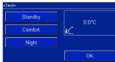
Since the room thermostat touch surface is an active button, a window with three further buttons "Standby", "Comfort" and "Night" opens when it is pressed. Each of these three buttons has a 1-bit communication object by default. The objects "Comfort/Standby", "Night" and "Frost/heat protection" are linked via a group address to objects with the same names in a room thermostat.
