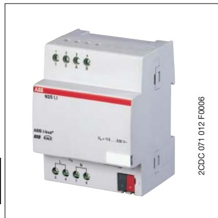
The Weather Unit WZ/S 1.1 is used for recording weather data – primarily for domestic purposes. The Weather Sensor WES/A 1.1 is connected to the WZ/S 1.1. The connection to the bus is established via the Bus Connection Terminal at the front of the device. The device is ready for operation after connecting the mains voltage of 115...230 V AC and the bus voltage.
