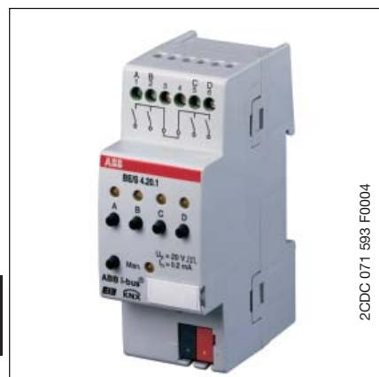
The 4-fold Binary Input BE/S 4.20.1 with manual operation is a rail mounted device for insertion in the distribution board. The device is suitable for reading out of floating contacts. The pulsed polling voltage is generated internally.
