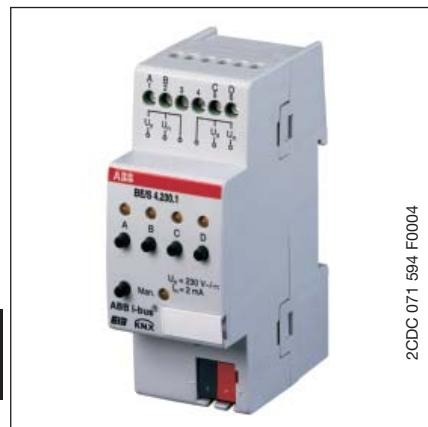
The 4-fold Binary Input BE/S 4.230.1 with manual operation is a rail mounted device for insertion in the distribution board. The device is suitable for reading out 0...265 V AC/DC signals. Inputs A and B are independent of inputs C and D.
