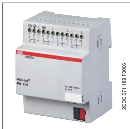
The Blower/Fan Coil actuator is a modular installation device in ProM design for installation in the distribution board on 35 mm mounting rails. The 2-fold Blower/Fan Coil actuator can control single phase ventilation, fans and fan coil units (2-, 3- or 4-pipe systems) with the application program "FanCoil, 2f 6A/1". The connection to the ABB i-bus® EIB / KNX is implemented via bus connection terminals.
