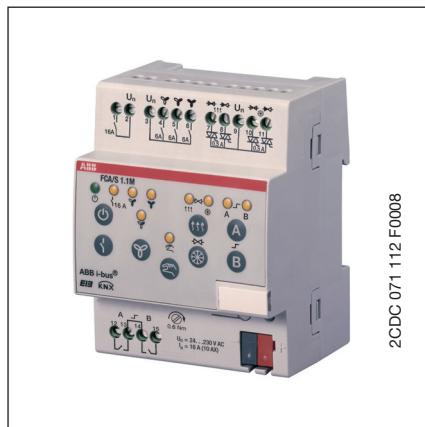
The Fan Coil Actuator FCA/S 1.1M is a modular installation device (MDRC) in proM design. It is intended for installation in the distribution board on 35 mm mounting rails. The assignment of the physical address as well as the parameter settings is carried out with ETS2 from version V1.3a or higher.
