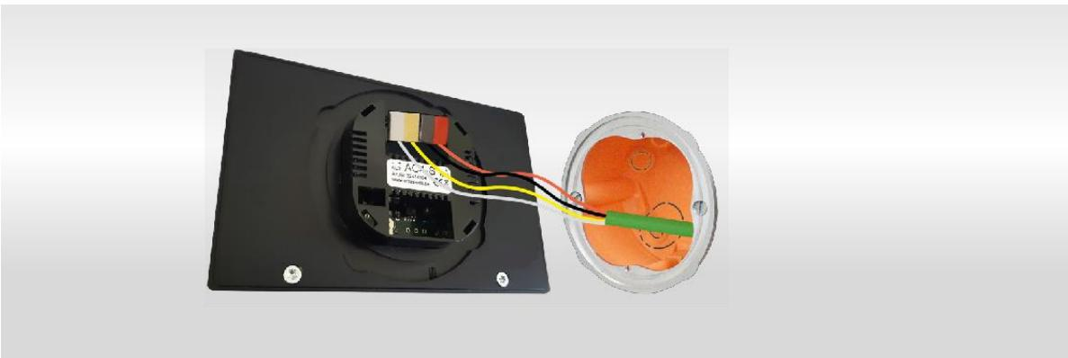
The display is designed for flush mounting. The degree of protection is IP20. It is mounted using the supporting ring, a locking screw type Torx-6 is used for fixing.
