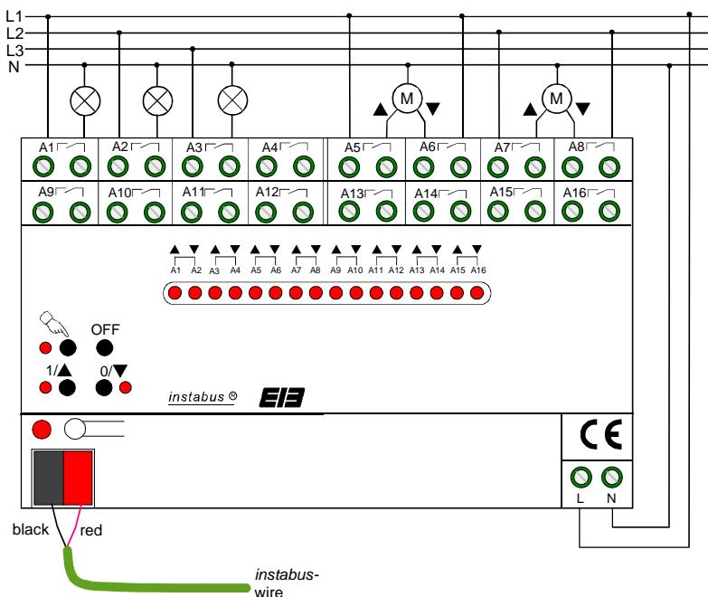
The mains voltage and the loads are connected as shown in the diagram above. The example shows connection of 3 lamps to outputs A 1 – A3 and 2 blind/shutter motors to outputs A5/A6 and A7/A8. Further loads are connected in the same way.
