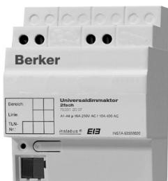
The Universal dim actuator 2gang operates according to the phase control or cut on principle and enables the switching or dimming of filament bulbs, high voltage halogen lamps as well as low voltage halogen lamps via conventional transformers and Tronic transformers. The unit automatically measures the properties of the connected load and sets the appropriate dimming procedure.
