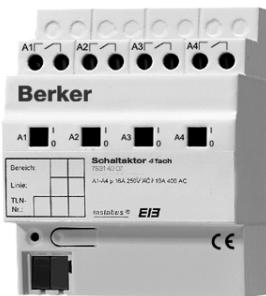
The switch actuator receives telegrams via the EIB and switches groups of electrical equipment with its four potential-free independent relay contacts. Various external conductors can be connected. The application enables switching with feedback (revertive signal), logic operation and timer function. The slide switches can be used to manually activate the 4 relays in parallel with the instabus EIB or to switch them on or off without the instabus EIB.
