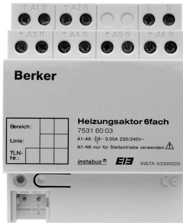
The heating actuator is for activation of electro-thermal actuator drives (ETA) for heating systems or cooling systems. It has 6 electronic outputs, which silently activate the actuator drives in response to EIB telegrams.
