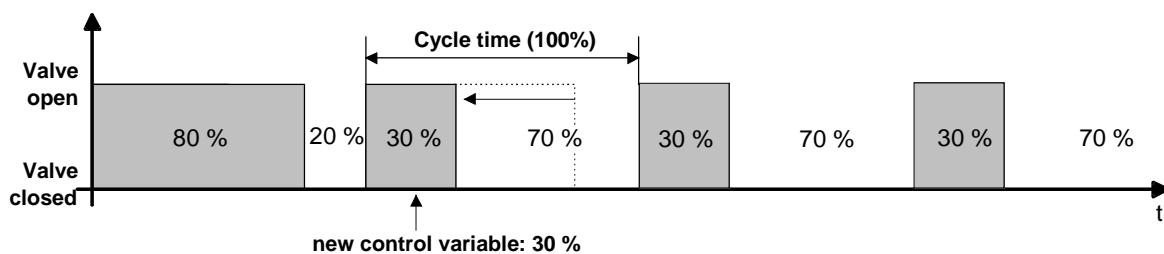
Before receipt of the new manipulated variable (30 %) the old setpoint (80 %) was active. The new manipulated variable is received during the opening phase of the valve. At this point in time the actuator recognises that it is still possible to cut short the opening phase so that it corresponds to the new manipulated variable (30 %). The cycle time is unchanged by this procedure.
