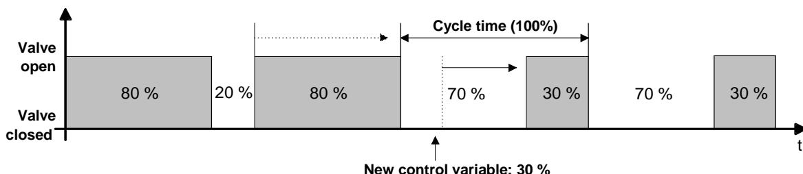
Before receipt of the new manipulated variable (30 %) the old setpoint (80 %) was active. The new manipulated variable is received during the closing phase of the valve. At this point in time the actuator recognises that it is still possible to cut short the closing phase so that it corresponds to the new manipulated variable (30 %). The cycle time remains unchanged, the starting time of the period is nevertheless automatically delayed.
