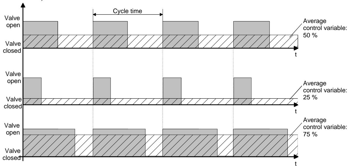
Based on the parameter "Mode of operation of valve / valve drive combination" for each output, the respective output is energised or not energised depending on the valve setting to be achieved.
