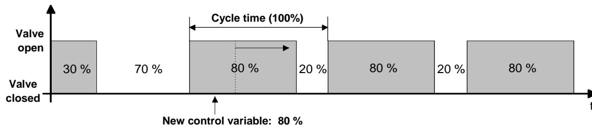
Before receipt of the new manipulated variable (80 %) the old setpoint (30 %) was active. The new manipulated variable is received during the opening phase of the valve. At this point in time the actuator recognises that it is still possible to extend the opening phase so that it corresponds to the new manipulated variable (80 %). The cycle time is unchanged by this procedure.
