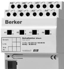
The switch actuator receives telegram via the EIB and switches groups of electrical devices with its eight potential-free, independent relay contacts. Various external conductors can be connected. The application enables switching with revertive signal (feedback), logic operation and timer function. The slide switches can be used to manually activate the 4 relays (outputs 1-4) in parallel with the instabus EIB or to switch them on or off without the instabus EIB.
