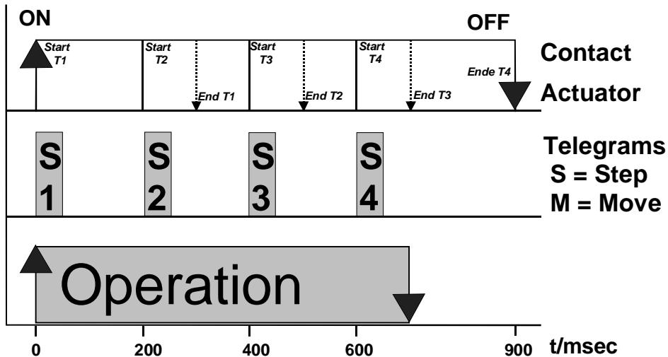
Functional sequence of the **shutter controller** with parameter settings:
