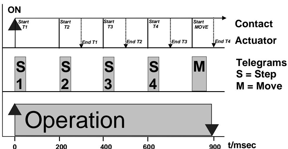
If the activation stops after transmitting all the stepped commands, then a continuous command (Move) will be transmitted to the bus controlling the actuator in lock mode according to the time in the parameters (factor x basis).
