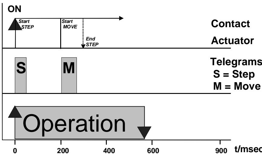
Functional sequence of the **shutter controller** with parameter settings:
