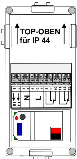
The 1 port shutter / 2 port switch actuator with extension input receives telegrams to control operating equipment. The type of operating equipment is defined based on the circuitry and the application software. The extension function allows internal and external control over conventional sensor elements. IP44 protection is achieved in surface-mounted installations that comply with the installation requirements.
