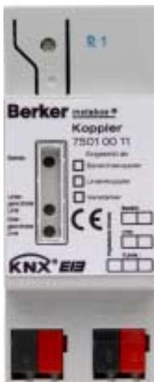
The area / line coupler connects two instabus EIB lines with one another to form a logical functional area and ensures electrical separation between these lines. Each bus line of an EIB installation can therefore be electrically independent of other lines.
