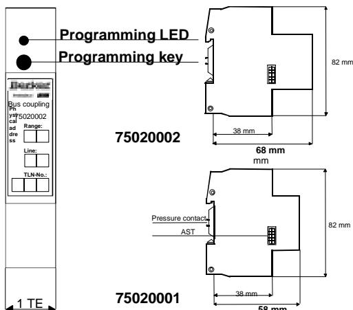
Logic controllers for series installation on DIN rails.
