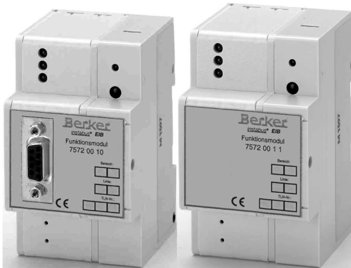
The function module is a maintenance-free, programmable controller for use in the EIB. As a supplement to the decentral system the extensive functions library can be used to solve various control and automation tasks. EIB telegrams from different EIS are received, processed and the results transmitted to the bus within a defined period. The function modules have an internal real-time clock which can be used both as a time switch and as a timer.
