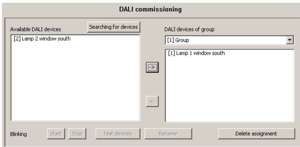
Figure 43: Assigning a device to a group
