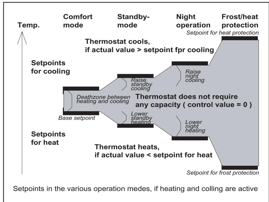
It is possible to preselect a setpoint for heat protection which enables the room to be cooled despite the window being open. If heat protection is not required, the cooling mode can be disabled. In this case, the receipt of an "On" telegram at the frost/heat protection object causes the value 51°C to be output via the setpoint object instead of the current setpoint. The display in the thermostat mode then indicates "OFF".
