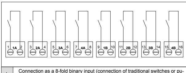
b Connection as a 8-fold binary input (connection of traditional switches or pushbuttons dedicated to the on/off switching of loads)
