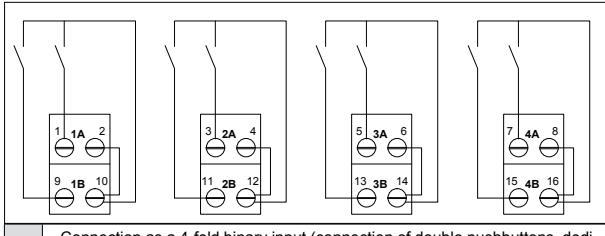
c Connection as a 4-fold binary input (connection of double pushbuttons dedicated to the control of dimmers or drives)
