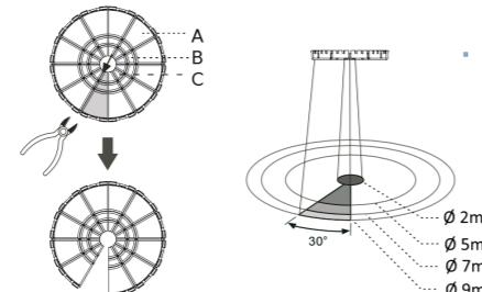
The device has degree of protection IP20, and is therefore suitable for use in a dry indoor environment. The device can be flush mounted through a 65 mm diameter hole on a ceiling board with 5 mm to 25 mm thickness; for solid ceilings, a plastic barrel-shaped plastic support for external mounting is available as an accessory.
