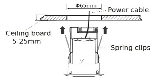
To remove the sensor, gently pry under the external rim with a screwdriver or another flat object; once you can get a firm hold with your hands on the rim, pull gently but firmly to extract the body of the sensor.
