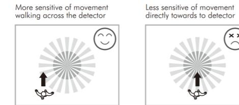
**i** The recommended mounting height varies from 2 m up to 5 m. Since the detector responds to temperature change, be aware that following conditions may cause lower sensitivity:
