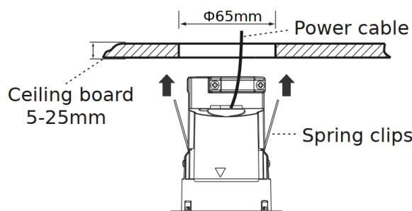
To remove the sensor, gently pry under the external rim with a screwdriver or another flat object; once you can get a firm hold with your hands on the rim, pull gently but firmly to extract the body of the sensor.
