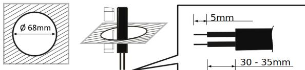
Drill a hole with Ø 68 mm on the ceiling
