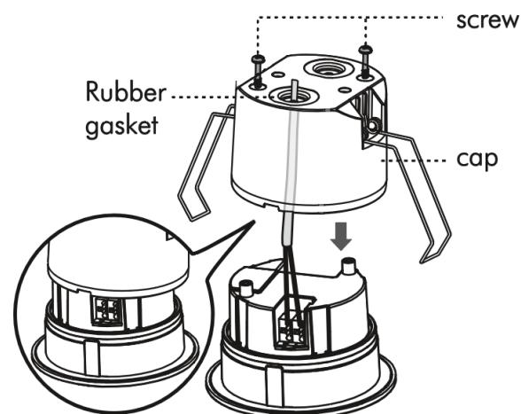
To insert the device into the hole on the ceiling board, raise and hold the spring clips; guide them into the hole and gently slide the body of the sensor until it falls into place.
