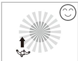
Less sensitive of movement directly towards to detector
