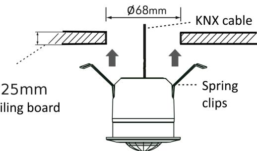
To remove the sensor, remove the bezel, gently pry under the external rim with a screwdriver or another flat object; once you can get a firm hold with your hands on the rim, pull gently but firmly to extract the body of the sensor.
