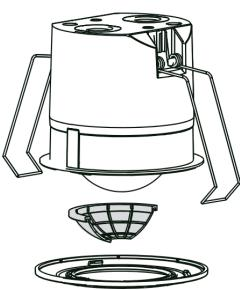
When the device is installed in place, make sure that the shield is in the correct position according to the required area masking.
