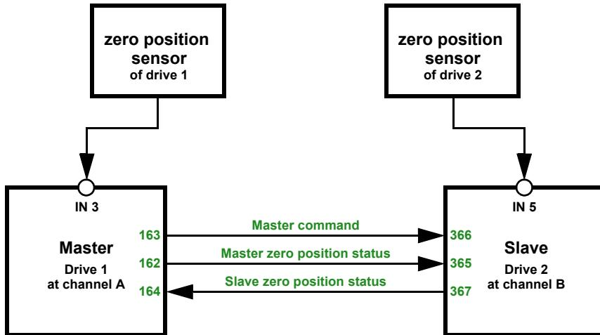
**Drive channel A is Master, zero position sensor at input 3 of the actuator, drive channel B is Slave, zero position sensor via bus:**
