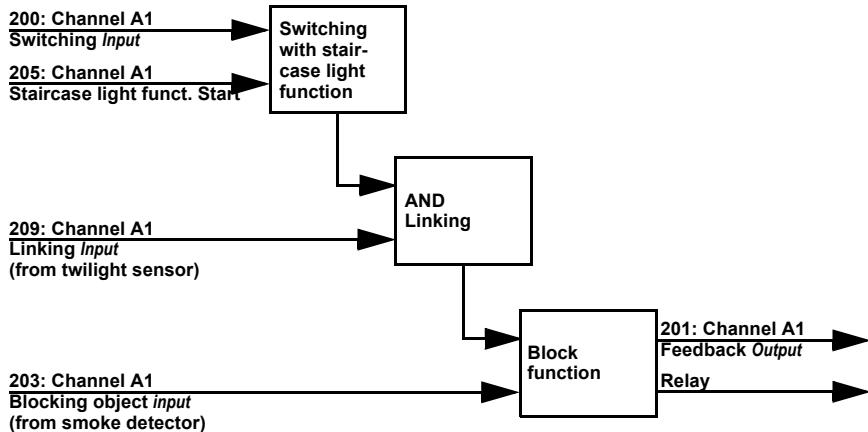
When switching via communication object "Channel A1 switch" (200), the light is turned on or off normally. When switching via object "Channel A1 staircase light function start" (205), the staircase light time function is activated. The time function has priority, i.e. the status triggered by normal switching is overwritten.
