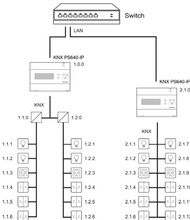
The physical address assigned to the KNX PS640+IP determines whether the device operates as a line or backbone coupler. If the physical address is in the form of x.y.0 (x, y: 1..15), the router operates as a line coupler. If it is in the form of x.0.0 (x: 1..15), the router acts as a backbone coupler.
