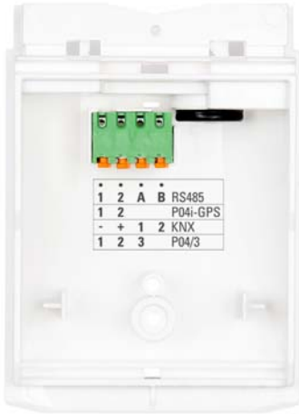
Fig. 13 Connect KNX data (+/-) and power supply (12...40V DC, 12...28V AC, 1|2) to the connector.
