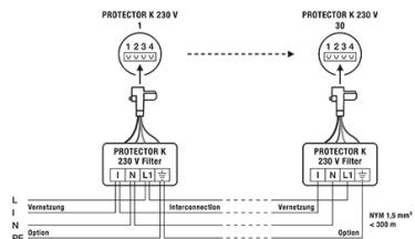
Connection 230 V ACSmoke detector PROTECTOR K 230 V filter
