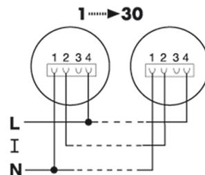
Connection 230 V ACSmoke detector PROTECTOR K 230 V filter
