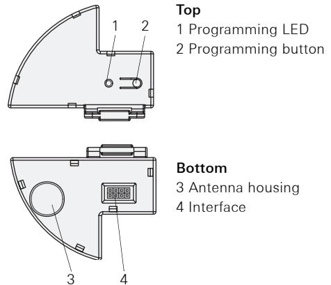
**Do not insert the radio module while the battery is connected**
