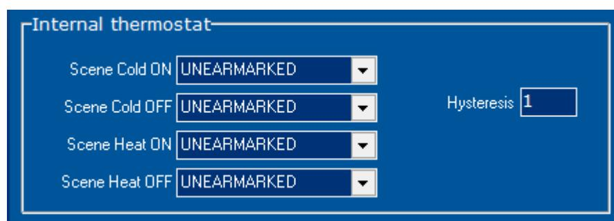
The hysteresis is the allowed difference between the set point value and the measured temperature, in other words, is the range within any order is sent. This parameter is used to avoid oscillations.
