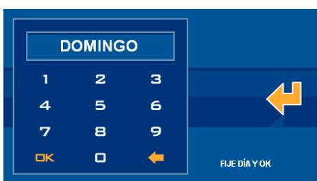
Note: When the device is disconnected from the power supply it is necessary to set the day and hour manually. If the installation incorporates the Ingenium RTC it is done automatically (see the RTC documentation for further information).
