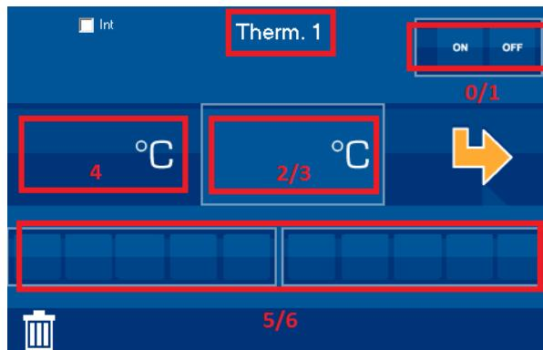
There are 10 programmable buttons that allow to control the working modes of the thermostat. They are restrictive by groups (left group and right group), it means that if one is activated the others are deactivated.
