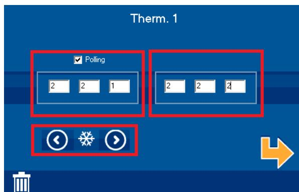
If the MEKBUS is working in conjunction with STIBUS-SD Ingenium model, the internal thermostat is programmed by selecting the corresponding tick:
