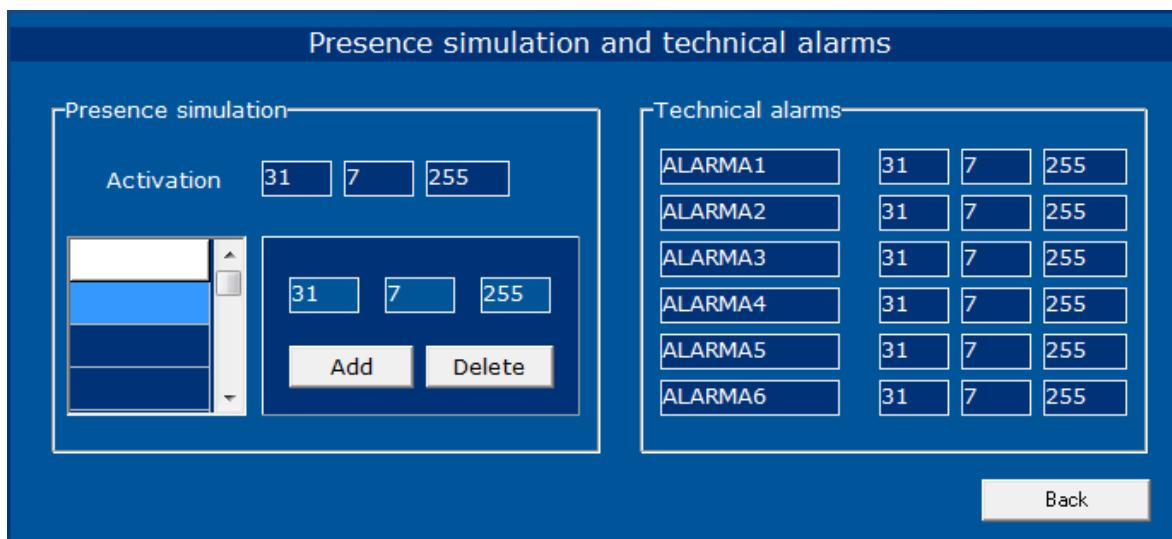
The MEKBUS incorporates a presence simulation function that allows to copy the last actions done by the customer and reproduces them as if there were people at home. In this configuration menu we have to set the group addresses that the screen will copy and the group address for activation and deactivation it remotely.
