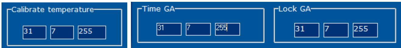
*Temperature calibration:* The temperature measured by the screen can be calibrated through this group address. To calibrate it with a reference thermometer proceed as follows:
