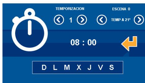
First, select the number of timing to use and the scene that will be scheduled (they must be programmed before) with left and right arrows in the top right corner of the screen. Then, press over the hour to set the hours and minutes of execution with the keyboard.
