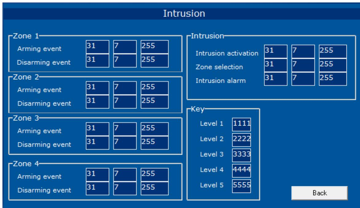
**Zones:** The MEKBUS can manage up to 4 intrusion zones sending a bit telegram to activate or deactivate any of them, these group addresses can be used to enable/disable the different sensors in the installation.
