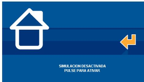
Press over this icon to show the presence simulation menu and activate it by entering any intrusion code and pressing ok with the keyboard.
