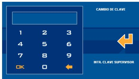
Then, select the level of password to be changed by pressing form 1 to 5 on the keyboard and enter the new one twice to confirm it. If the level selected is 5, you will change the administrator code.
