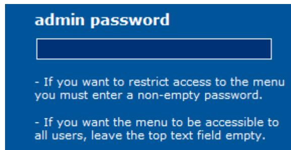
This function is enabled just by writing a password. If the menu is blocked (administrator mode enabled), press in the centre of the Smart Touch main window for 5 seconds approximately and use the keyboard to enter the access password.
