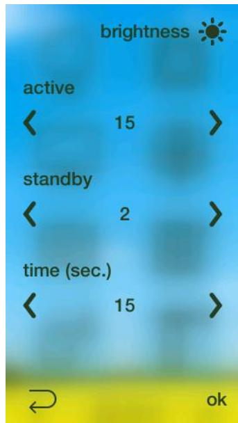
Active [3 - 15]: Is the brightness level when the screen is being used.
