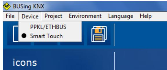
When the target of the project is a Smart Touch, it must be selected in the corresponding menu: Device -> Smart Touch.
