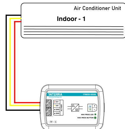
The figure on the right shows the connection diagram between the LG AC-KNX Gateway and single air conditioner indoor unit.
