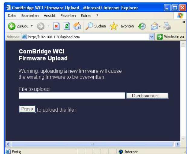
Select the upgrade file via the "Search" button and load it into the device by pressing the button "Press". Update files have the following name:
