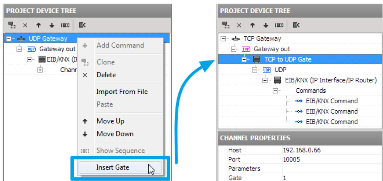
As a result you get a new level in the Device Tree (TCP Gateway) where you can set the connection of iRidium Client to the iRidium Gate server for transferring data to the addresses of the lower level (UDP Gateway) which are indicated when setting up the operation in the local network.
