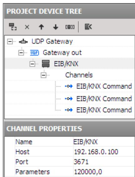
For setting up of the connection to the KNX IP-router you should indicate the IP-address of the router, UDP connection port (it is always 3671 for KNX/EIB) and Time-out (ms) of the connection at the loss of communication.
