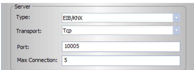
Device (connection properties of the Gate application to the equipment of the KNX/EIB bus):
