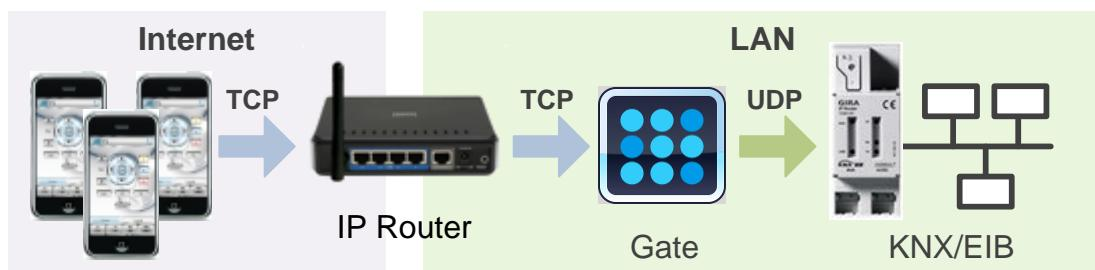
Capabilities of the iRidium Gate bus for KNX/EIB: suppose that you use a JUNG IPR 100 REG IP Router to control the KNX equipment. There are some limitations when using such type of connection:
