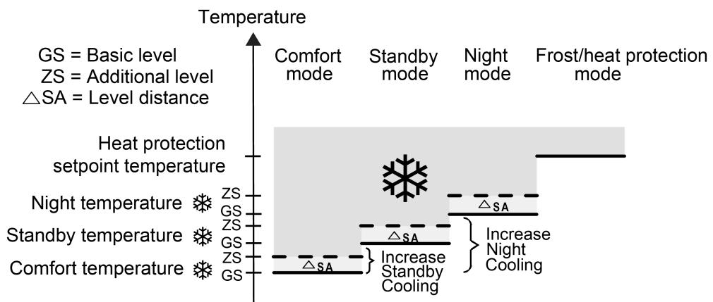
Figure 63: Setpoint temperatures in the operating mode "Basic and additional cooling"
