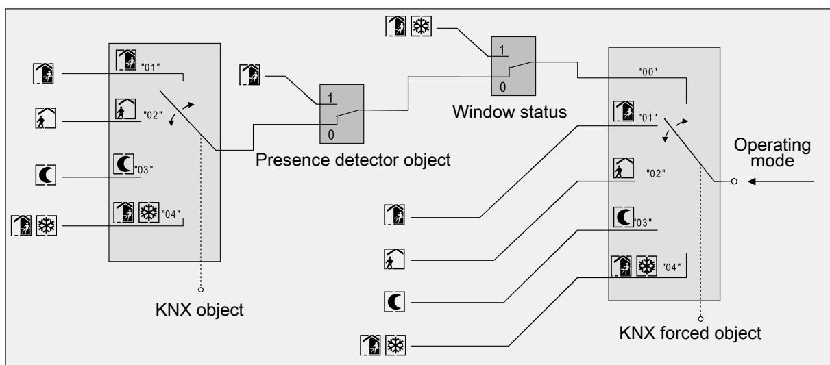
Figure 59: Operating mode switchover through KNX object with presence detector
