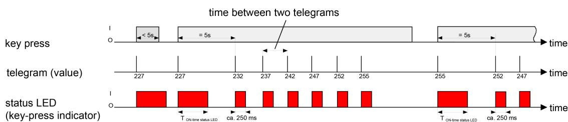
Figure 44: Example of value adjustment without value range overflow
