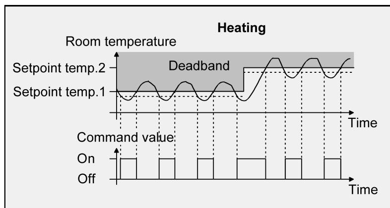
Figure 55: 2-point feedback control for mixed "Heating and cooling" mode with active heating mode
