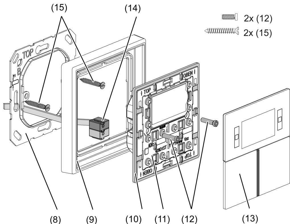
Figure 3: Mounting the controller module
