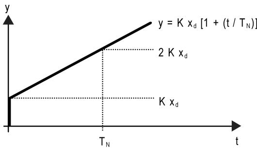
Figure 52: Function of the command value of a PI control
