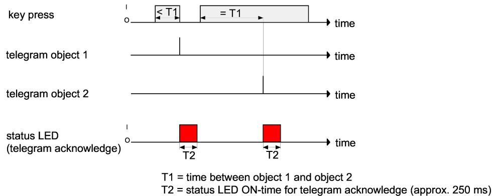
Figure 46: Example of "object 1 or object 2" operating concept
