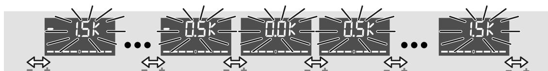
Figure 20: Setting the setpoint shift
