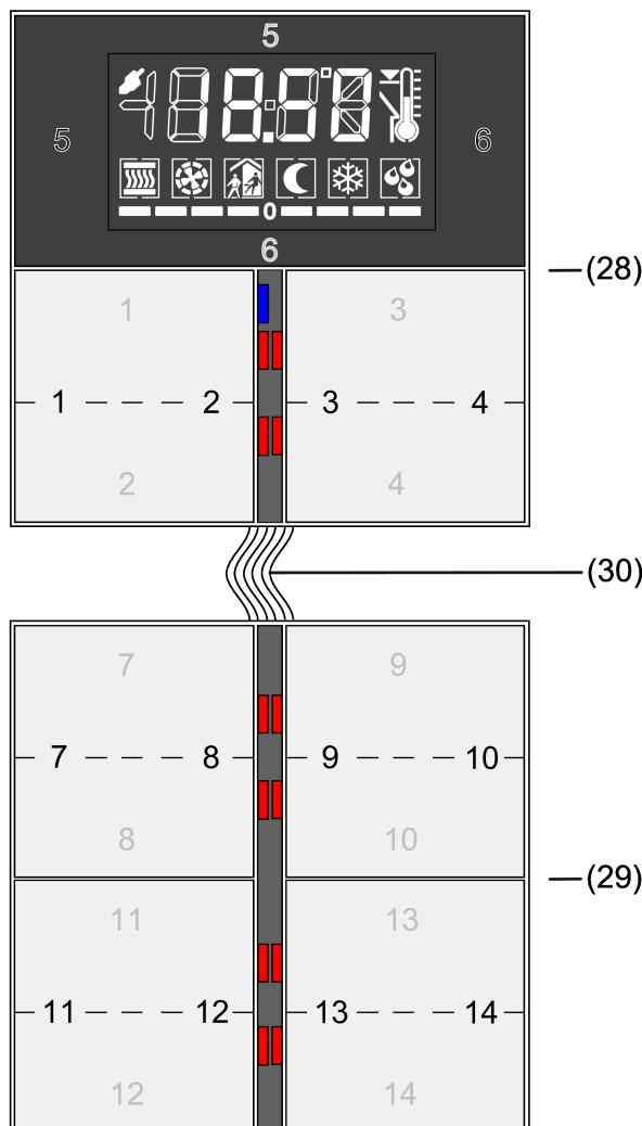
Figure 31: Example of button pair / operating area numbering in connection with a
