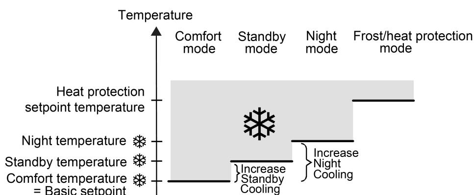
Figure 62: Setpoint temperatures in the operating mode "Cooling"
