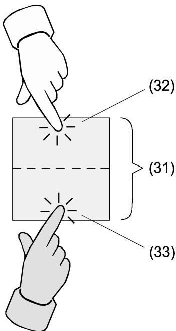
Figure 32: Example of rocker actuation
