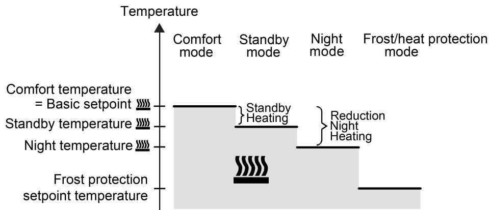
Figure 60: Setpoint temperatures in the operating mode "Heating"
