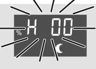
and the brightness value of the reduced backlighting are shown in the display. The push- buttons + and - can be used to adjust the brightness of the display in the range from 0 to 100%. The brightness reduction is only visible if the parameter "Brightness reduction" was activated on the "General" parameter page.
