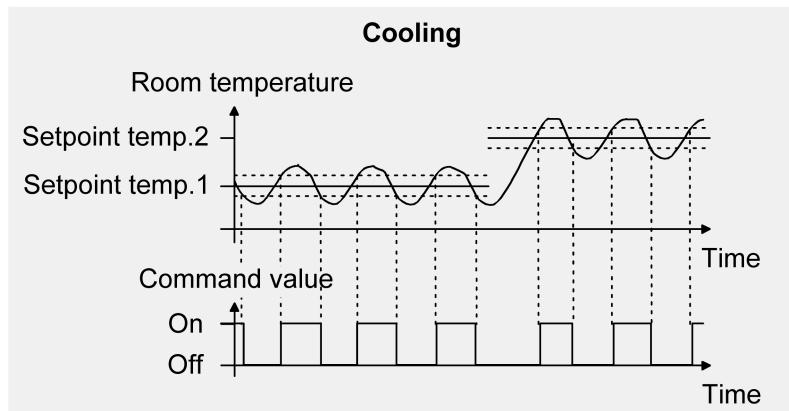
Figure 54: 2-point feedback control for the single "Cooling" operating mode
