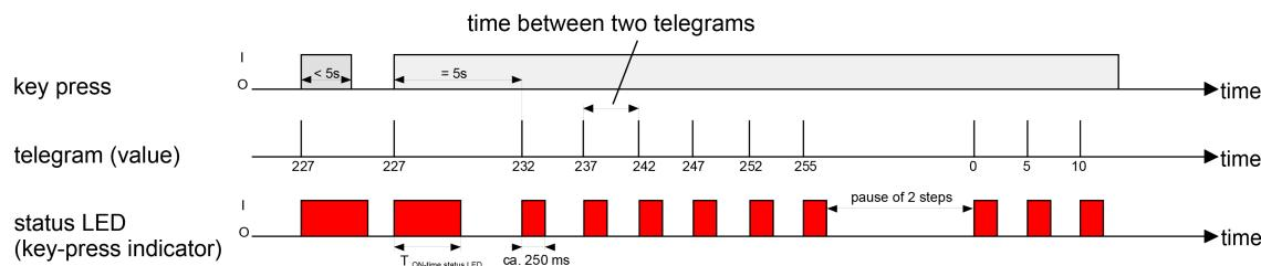
Figure 45: Example of value adjustment with value range overflow
