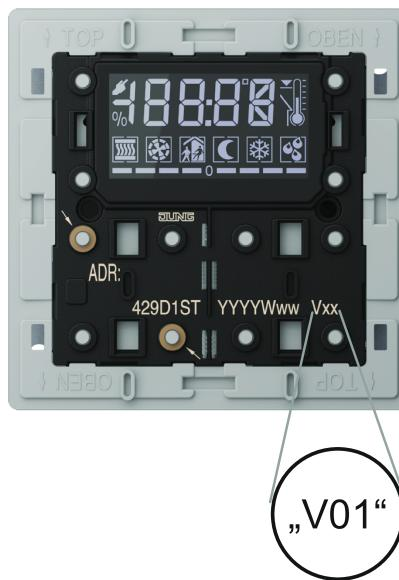
Figure 39: Designation of the device generation on the device
