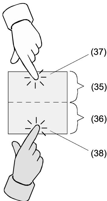
Figure 34: Example of button actuation with dual-area operation
