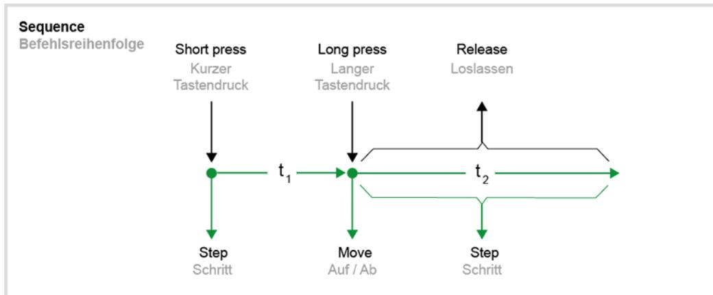
Figure 40: "Step - Up/down - Step" operating concept
