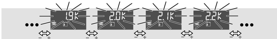
Figure 16: Setting the setpoint temperature increase for standby mode cooling
