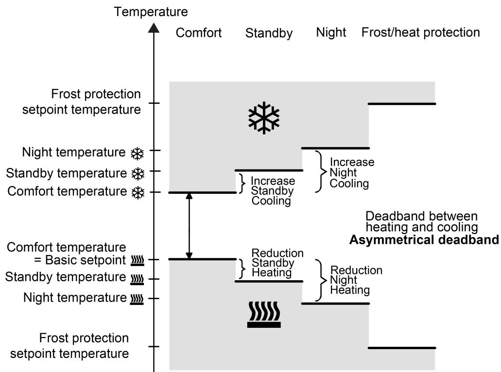
Figure 65: Setpoint temperatures in the operating mode "Heating and cooling" with asymmetrical deadband
