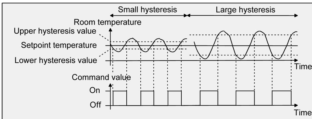
Figure 57: Effects of the hysteresis on the switching behaviour of a 2-point feedback control command value
