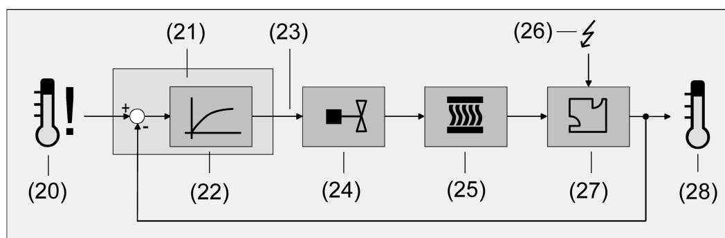
Figure 50: Controlled system of single-room temperature control
