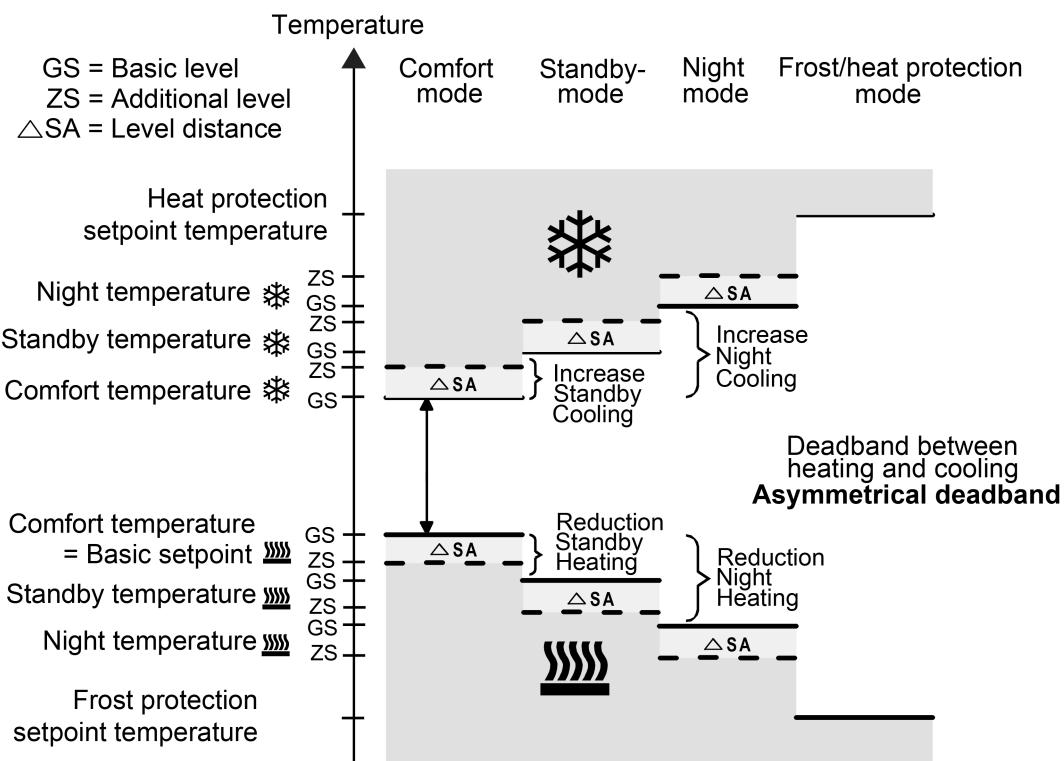
Figure 67: Setpoint temperatures in the operating mode "Basic and additional heating and cooling" with asymmetrical deadband
