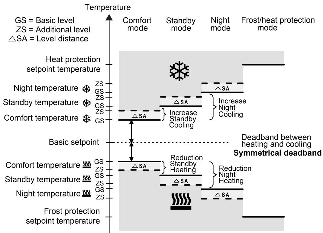
Figure 66: Setpoint temperatures in the operating mode "Basic and additional heating and cooling" with symmetrical deadband
