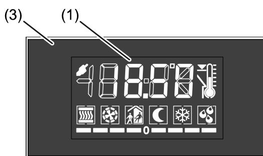
Figure 48: Device display and display operating element
