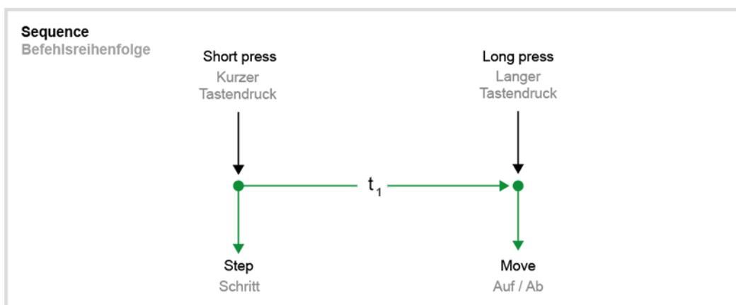
Figure 42: "Step - Up/down" operating concept
