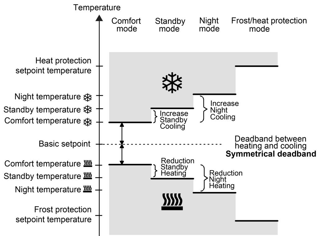
Figure 64: Setpoint temperatures in the operating mode "Heating and cooling" with symmetrical deadband
