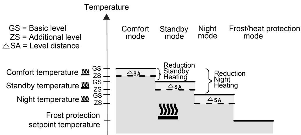
Figure 61: Setpoint temperatures in the operating mode "Basic and additional heating"
