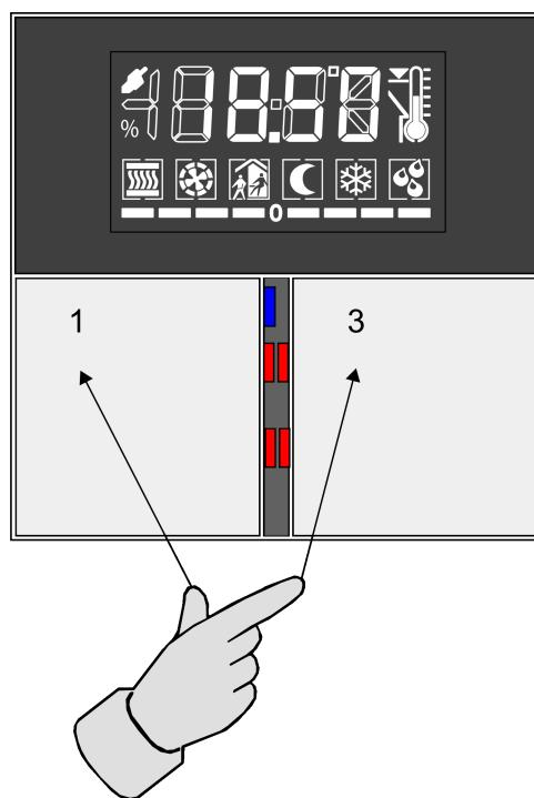
Figure 8: Button combination to recall the menu level
