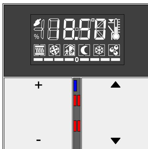
Figure 9: Button assignment for operation of the menu level
