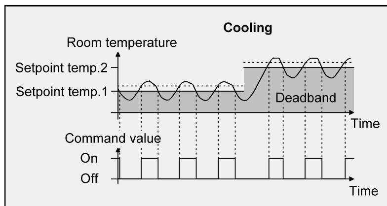
Figure 56: 2-point feedback control for mixed "Heating and cooling" mode with active cooling operation
