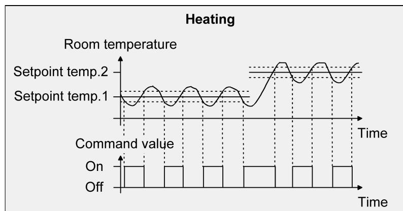
Figure 53: 2-point feedback control for the single "Heating" operating mode
