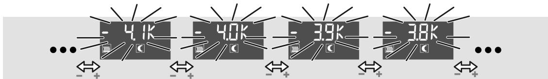
Figure 17: Setting the setpoint temperature reduction for night mode heating
