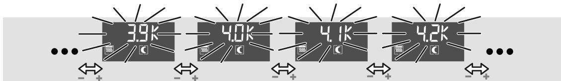
Figure 18: Setting the setpoint temperature increase for night mode cooling
