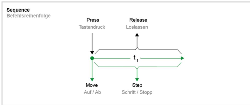
Figure 41: "Up/down - Step" operating concept
