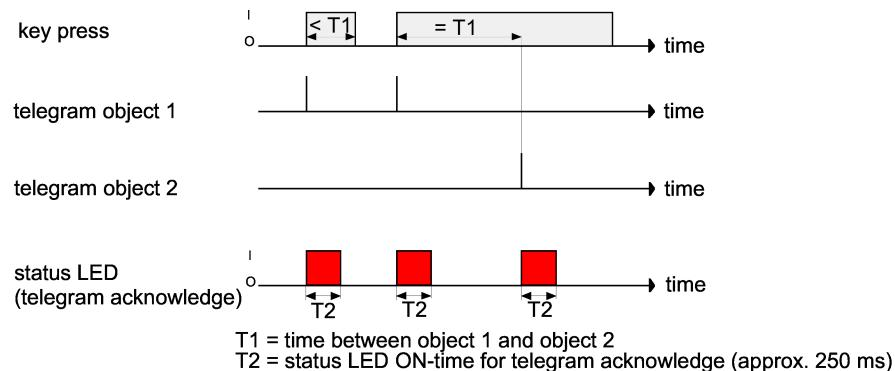
Figure 47: Example of "object 1 and object 2" operating concept
