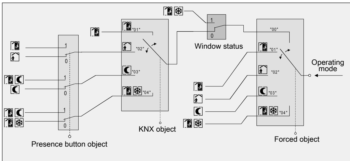
Figure 58: Operating mode switchover through KNX object with presence button
