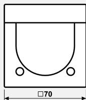
**IP** Protection level IP 44 is ensured with sealing kit ref.-no. AS CD 50 DS and "IP 44 frame" of the respective design range.
