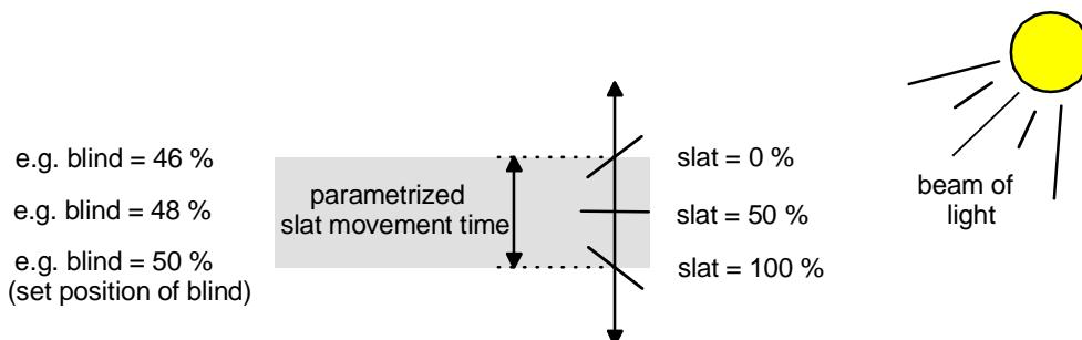
This example shows that slat angle changes result in a new blind position which is also followed up in the positioning objects. If the actuator receives in this case a 'new' blind position of e.g. 47 %, the actuator does not induce a movement, as the computed moving time falls into the parameterized slat moving time and thus coincides with the slat movement. A change of the blind position to 55 % in this example induces a blind movement as the change lies beyond the slat movement (0 to 100 %).
