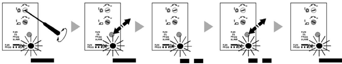
–: min. 1 s      Push RUN/PROG button briefly (< 1 s)      LED flashes      Push RUN/PROG button briefly (< 1 s)      LED is illuminated
