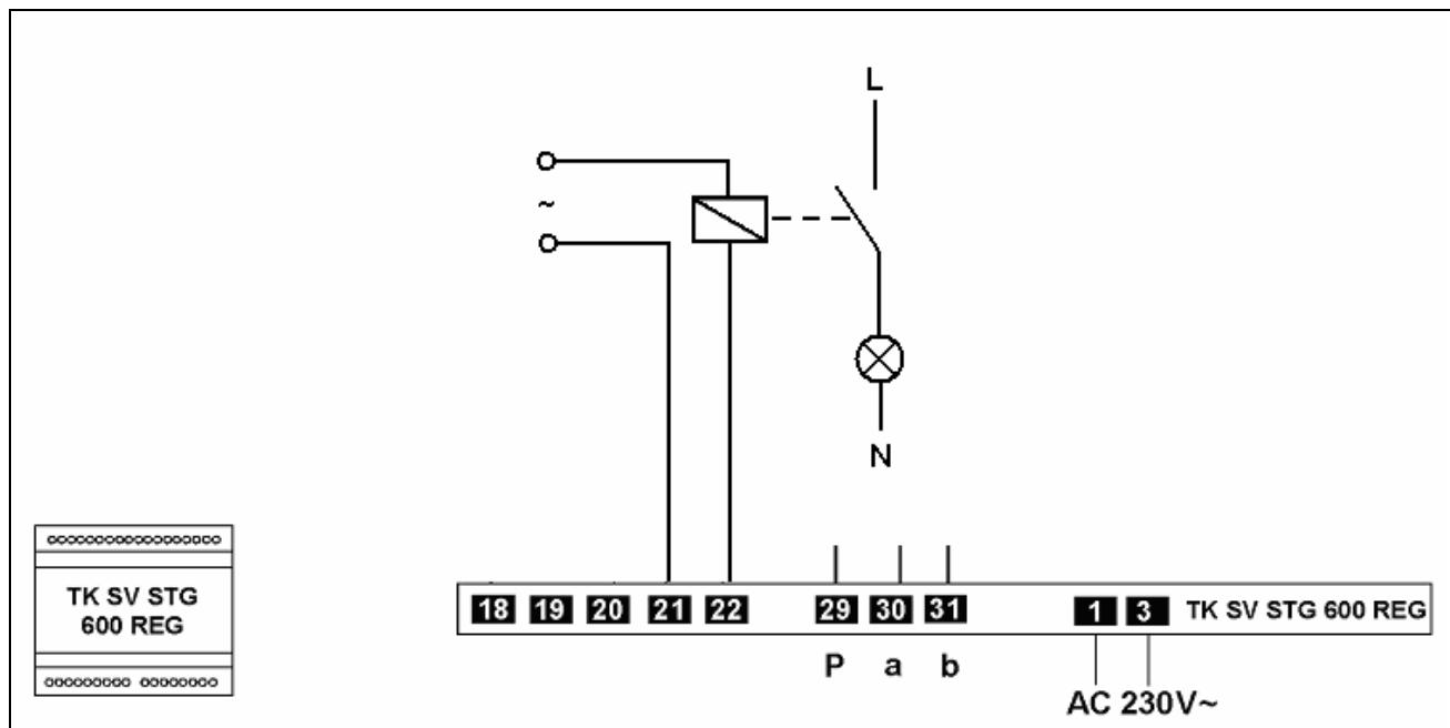
In an existing staircase installation, the switching contact of the *TKSVSTG 600 REG* has to be connected to the push-button terminal of the existing staircase timer switch. The light switching time has to be set to the minimum at the power supply & control unit.
